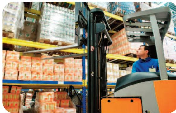
confirming that the forklift is safe to drive, by an authorised operator, questions such as “Are you wearing appropriate PPE?” or “Are you under the influence of any medication?” can be included to reinforce the message that operating a potentially dangerous piece of equipment is not to be taken lightly.
